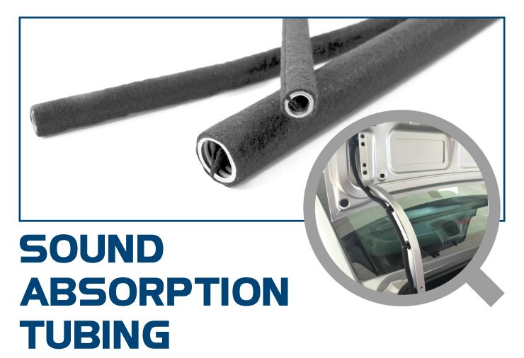
The SOUND ABSORPTION TUBING combines the mechanical protection of a regular convoluted tube and the dampening properties of a polyester felt.
